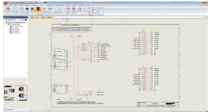
With the improved accuracy afforded by SOLIDWORKS Electrical 3D, GLSV has reduced electrical cabinet sizes to what’s actually necessary, helping the company satisfy customer demand for smaller footprints.
